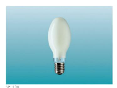
Single ended, high pressure Mercury vapour lamps consisting of a gas-filled soft glass phosphor coated outerbulb. The arc-tube is filled with mercury amalgam. The new HPL 4 Pro lamp achieves maximum light output and peak luminous efficacy at temperatures as low as 15°C, around the lamp. They are therefore particularly suitable for use in outdoor applications especially for those where group replacement costs have a large influence in descision making.
